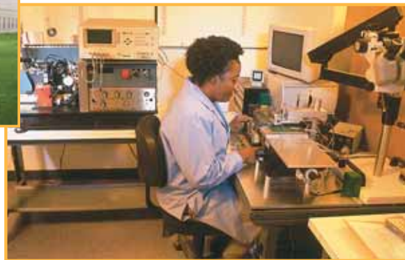
▶ Autopacking center packages chips into waffle packs
