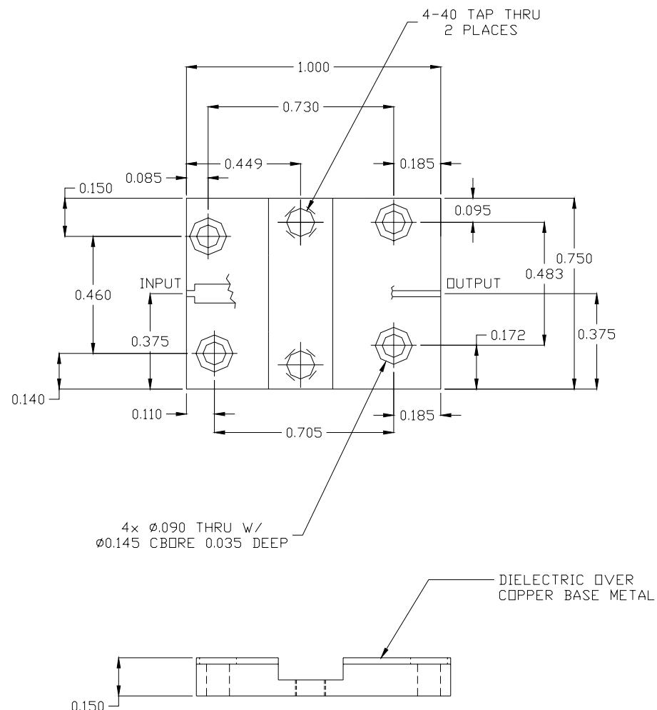
**50Ω RF TEST FIXTURE**
